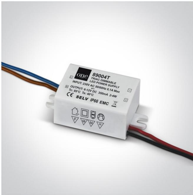
IP66 Constant current LED driver, Triac dimmable, for 350mA LED spots / LED fittings, 2-4W.
