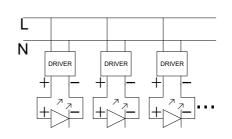
\* The number of modules that can be connected in series depends on the available output voltage of the LED driver.
