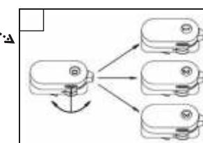
Four line three circuit for track adapter. The fixture adaptar can be used on 0,1,2 and 3 circuit track system. An adjustable contact on the fixture adaptar allows you to select the circuit position.
