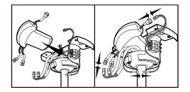
Wire up the receiver with quick connectors and insert into the mounting bracket. Make sure the antenna wire has been safely folded inside the canopy cover before final assembly. (DO NOT cut the antenna wire)
